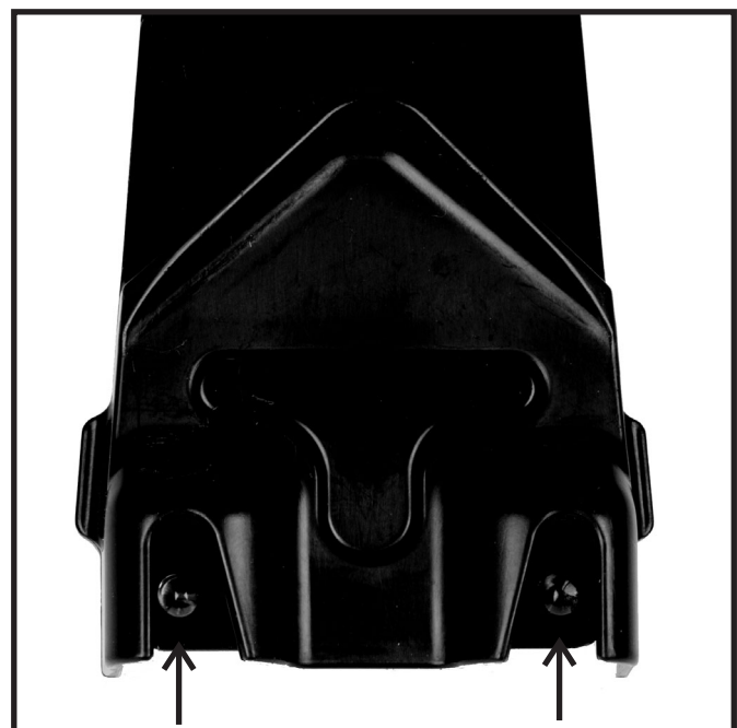
Photo-Eyes in New Ice Sensor
